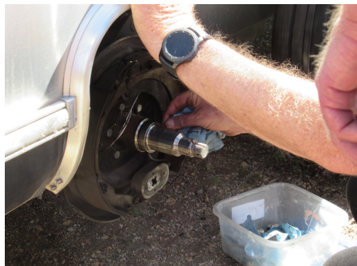
Clean Spindle Ready for Fresh Grease & Bearing
