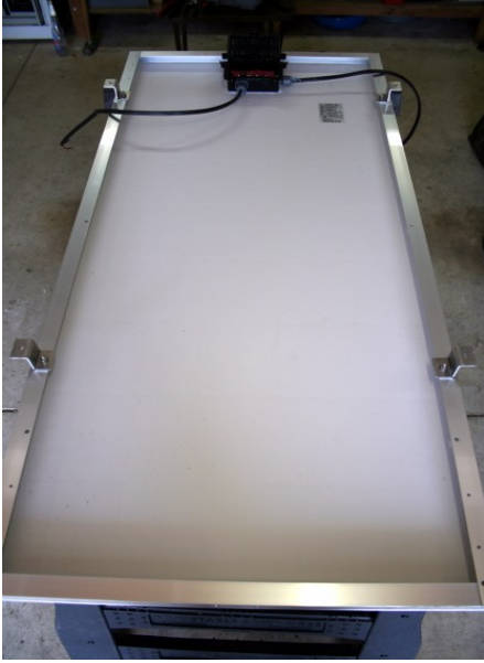
1: PV Panel with Wiring (Note Relocated Lower Mounts)
