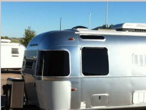
New Airstream with raised center roof panel for a/c ducts
